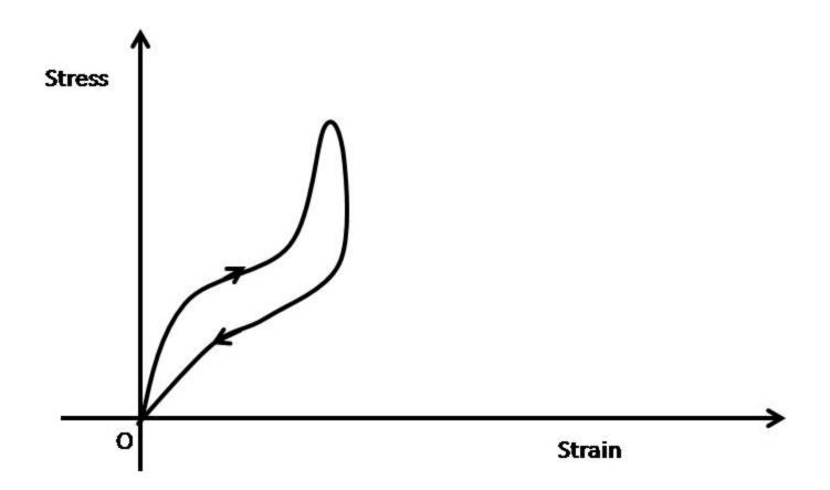
The lack of coincidence of the curves for increasing and decreasing stress is known as elastic hysteresis. The area of the hysteresis loop is proportional to the energy (per unit volume) dissipated within the elastic material.
